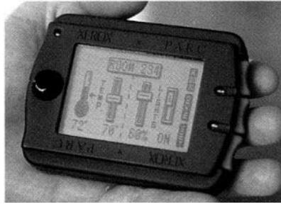
A PARC Tab handheld computer being used to adjust office temperature and lights.
